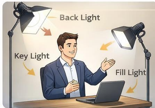
Gambar 41. Skema Three-Point Lighting
